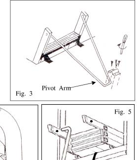
Fitting the handrail Engaging the operating pole
