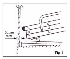
2. Slide ladder along base so that the plastic feet are overhanging the edge of the loft floor. With assistance (if required) release catches on side of ladder and lower section to the floor.
