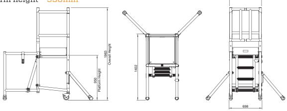
Maximum Safe Working Height\*: 2.95m Maximum Safe Working Load: 150kg
